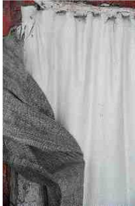
Figure 8. Fabric 'curtain' made from Fabric Formwork, Mark West
