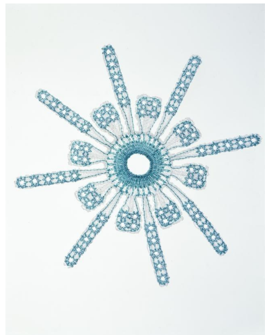
Figure 10. Machine embroidered Bio implantable device for reconstructive shoulder surgery, Professor Simon Frostick
