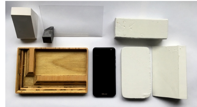
Figure 4: Components of Design Daydreams augmented post-it notes (clockwise from top left): carved wooden holder, 45 degree wedge, transparent film with concrete corner weight, simple 3D shapes on which to overlay images, mobile phone
